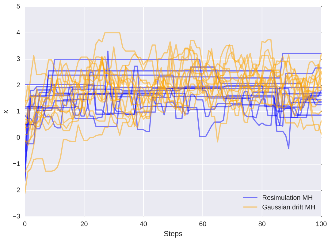
Figure 4.6: Top: A VentureScript program that uses a custom user-defined inference procedure (shown in Figure 4.7) for random-walk MH with Gaussian drift proposals. Bottom: A plot comparing sample trajectories of the Markov chain obtained from this inference program with sample trajectories from the program in Figure 4.4 which uses independent resimulation proposals. The Gaussian drift proposal is accepted more frequently, suggesting that the custom sampler is more efficiently exploring the space of traces.
